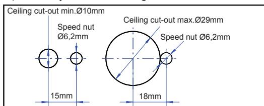
According to the ceiling cut-outs, in a distance (middle hole ceiling cut-out – middle hole captive nut) of at least 15mm and max. 18mm next to the ceiling cut-out you drill a hole for the speed nut. A speed nut for sheet metal ceilings and a screwed insert for wooden ceilings are included in the scope of delivery.
