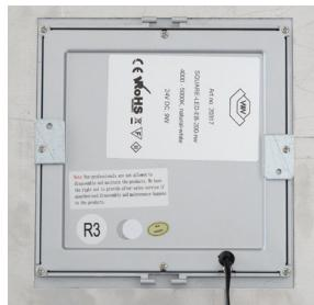
Loosen the screws holding the fixation plates of the lamp. Turn the fixation plates towards the outer edge of the lamp, so that the chamfered sides of the fixation plates face outward. Tighten the supporting screws of the fixation plates again. Lock the lamp into the sheet metal plate of the ceiling by screwing the supplied M4x16 screws into the open holes of the fixation plate, until the screws sit tightly on the sheet metal plate. Mount the intermediate ceiling.
