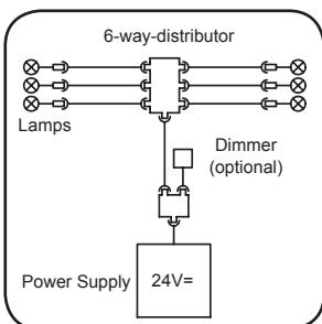
Please provide for a 12mm cable feedthrough for the line connecting the 6 way distributor and the power supply unit at a suitable position in the cabin ceiling towards the cabin roof. Therefore use the enclosed rubber cable duct. The power supply unit should not be placed in the cabin ceiling.
