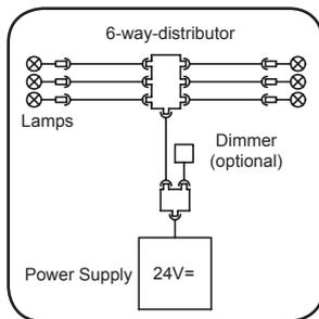
Please provide for a 12mm cable duct for the line connecting the 6 way distributor and the power supply unit at a suitable position in the cabin ceiling towards the cabin roof. Therefore use the enclosed rubber cable duct. The power supply unit should not be placed in the cabin ceiling.
