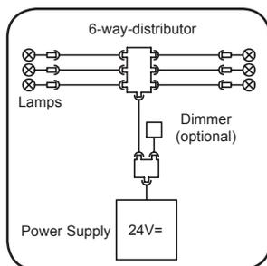
Please provide for a 12mm cable for the line connecting the 6 way distributor and the power supply unit at a suitable position in the cabin ceiling towards the cabin roof. Therefore use the enclosed rubber cable duct. The power supply unit should not be placed in the cabin ceiling.
