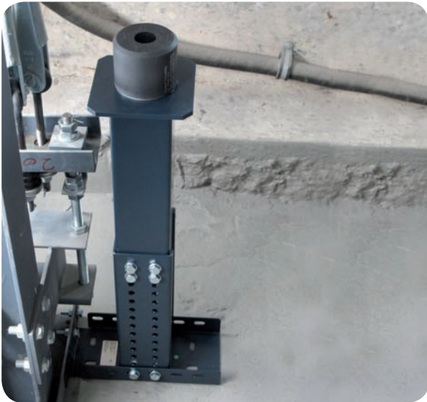
Mounting examples: buffer support size 3 with buffer
