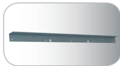
Sheet metal angle, galvanised, 28 x 28mm, t=1mm with holes for fastening with tapping screws, suitable for above-mentioned perforated sheet metal panels of 8 x 8mm.
