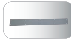
Sheet metal connecting plates, galvanised, width 60mm, t=1mm with holes for fastening with tap- ping screws, suitable for above- mentioned perforated sheet metal panels of 8 x 8mm.
