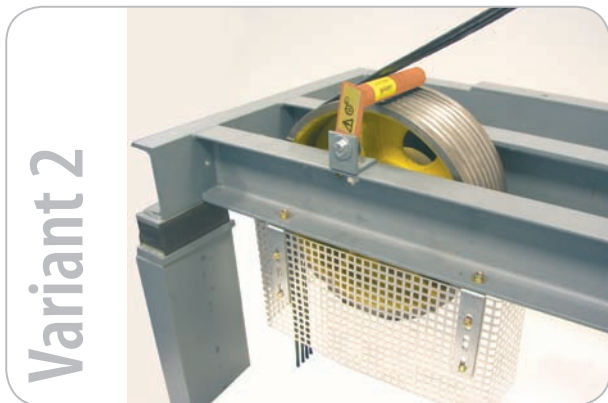
Mounting example of finger protection variant 2 , if the diverter pulley top is max. 100mm above the engine frame.
