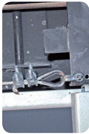
C Fixation cord at landing door - carriage
