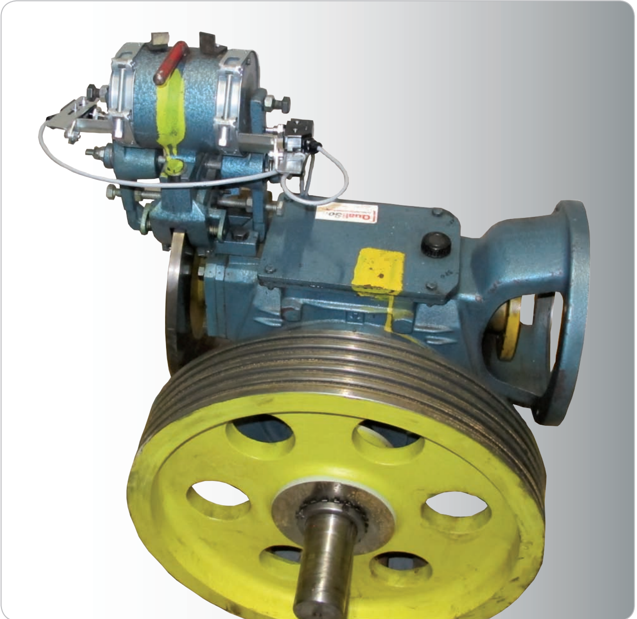
Mounting example brake monitoring on an old drive
